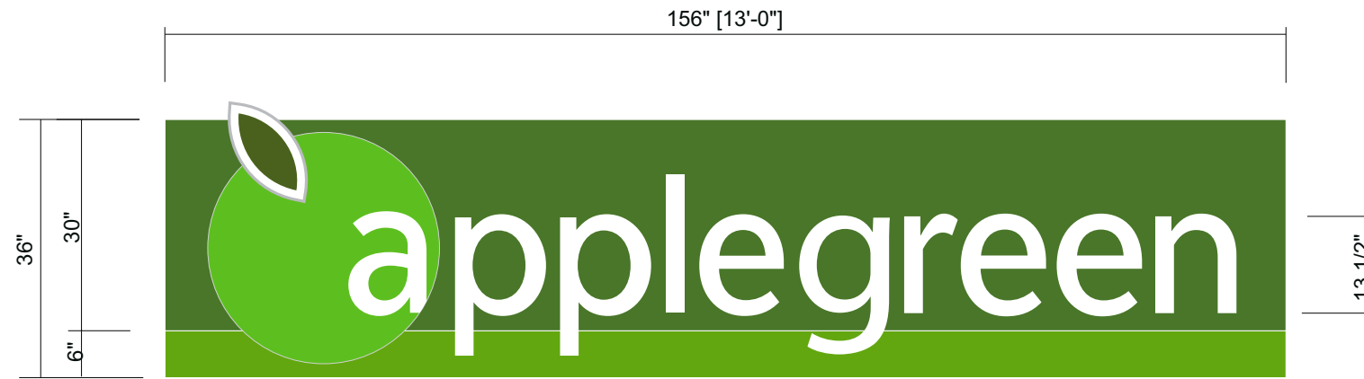
CHANNEL LETTERS FASCIA DETAIL (2) REQUIRED
